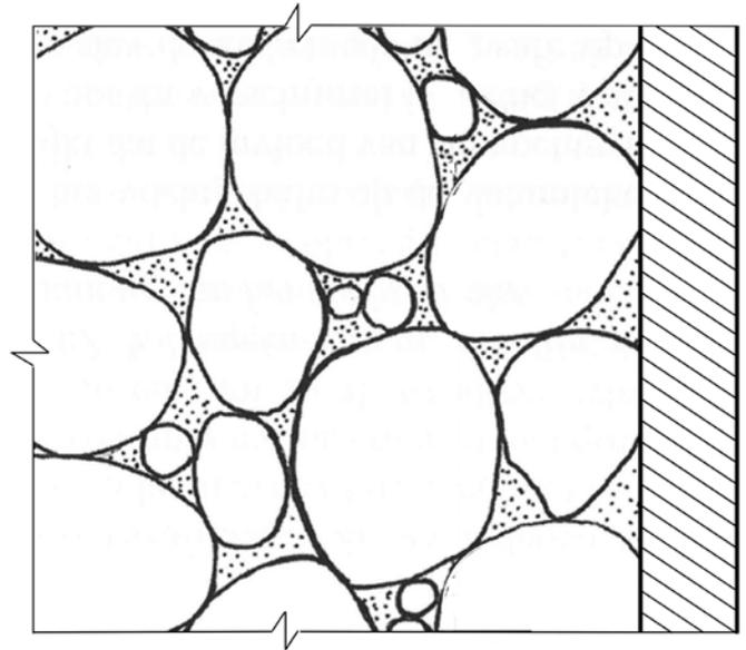
Fig. 4: Wall effect, based on Sourwerbreñ<sup>8</sup>
