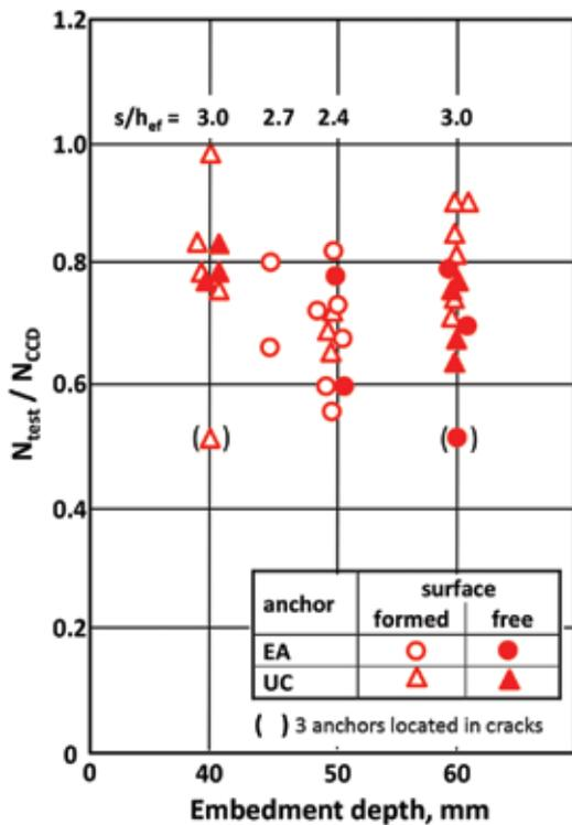
Fig. 10: Results of tensile tests on four-anchor fastening groups, showing the ratios of anchor group test capacities and capacities predicted using the CCD-method as functions of embedment depth. In this series, EA and UC were embedded in formed and troweled surfaces. For all but two cases, two out of four anchors were located in cracks, from Fuchs<sup>15</sup> (Note: 1 mm = 0.04 in.)
