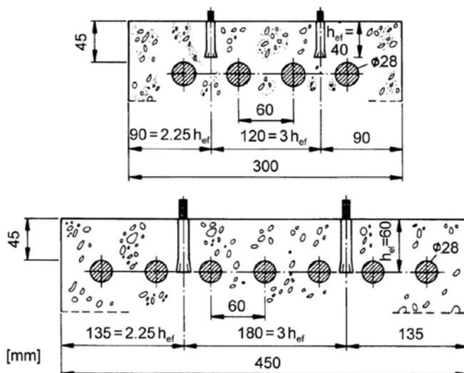
Fig. 8: Examples of anchorages in concrete cover of beams with heavy reinforcement tested by Fuchs<sup>15</sup> (Note: 1 mm = 0.04 in.)
