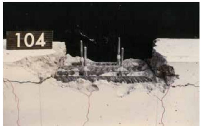
Fig. 9: An example of spalling of the concrete cover of a beam with heavy reinforcement and a quadruple fastening comprising expansion anchors subjected to tension load.<sup>15</sup> Note that the anchors were placed in their initial locations for the photograph
