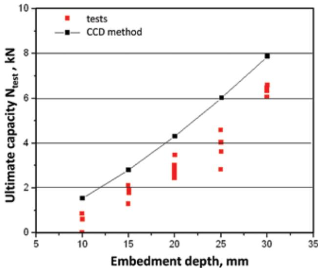
Fig. 12: Ultimate loads from tests in cracked concrete (25 MPa [3600 psi]) with a crack width of 0.35 mm (0.014 in.) as a function of the embedment depth in comparison to the values predicted according to the CCD-method,<sup>13</sup> based on Hofmann et al.<sup>16</sup> (Note: 1 kN = 224 lb; 1 mm = 0.04 in.)
