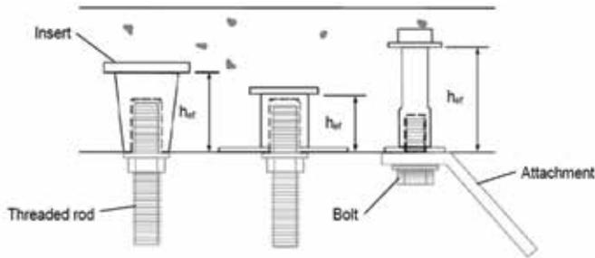
Fig. 2: Examples of cast-in specialty inserts covered by ICC-ES AC 446<sup>2</sup>
