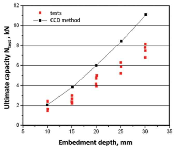
Fig. 11: Ultimate loads from tests in uncracked concrete (25 MPa [3600 psi]) as a function of the embedment depth in comparison to the values predicted according to the CCD-method, after Hofmann et al.<sup>16</sup> (Note: 1 kN = 224 lb; 1 mm = 0.04 in.)
