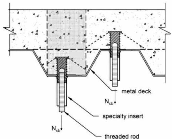
Fig. 6: Inserts in the soffit of concrete on deck assemblies with idealized concrete break-out body—examples from ICC-ES AC446<sup>2</sup>
