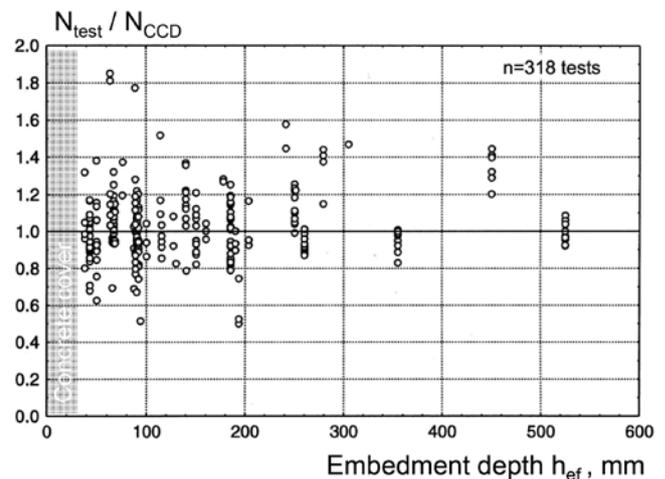
**Fig. 7: Results of tests that served as the basis for the development of the equation for determination of the concrete break-out strength of single headed anchors subjected to tension according to the CCD-method (Reference 13)**
