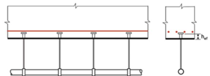
**Fig. 1: Anchorage of nonstructural loads with shallow embedded anchors. This example shows a redundant system with four individual anchors**
