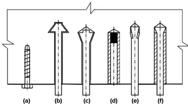
Fig. 3: Examples of mechanical post-installed anchors (after EN 1992-4<sup>5</sup>): (a) concrete screw; (b) undercut anchor, type 1; (c) undercut anchor, type 2; (d) drop-in anchor; (e) wedge type expansion anchor; and (f) sleeve type expansion anchor
