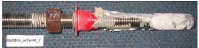
**Fig. 2: End-cap installation with voids (Ocel et al.<sup>7</sup>)**
